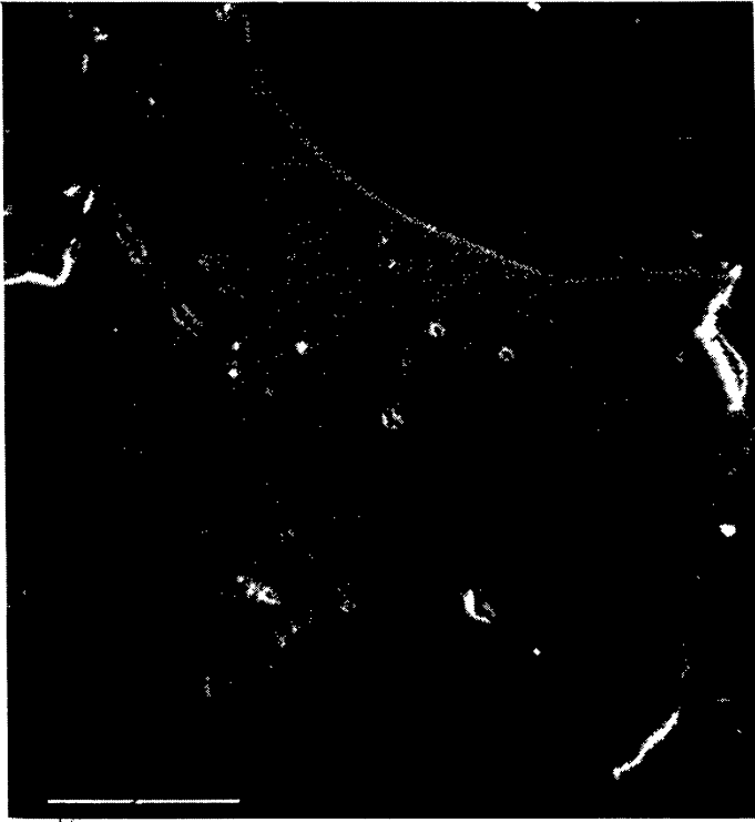
Fig. 4 Euhedral magnetite (M) embedded in interstitial pyrrhotite (S) between silicates (scale bar = 30 \mu\text{m} ).
