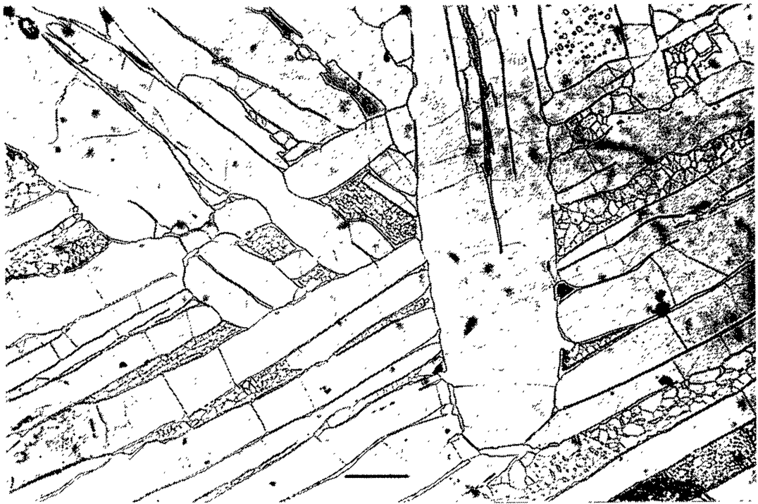
Fig. 7 Kamacite lamellae with Widmanstätten pattern, and small fields of cellular plesite. Reflected light after etching (scale bar = 150 \mu\text{m} ).
